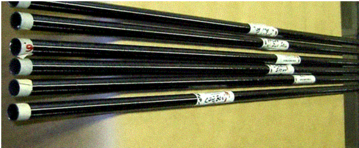
Figure 9-7 A picture of the first full length (1.5m) prototype Cerenkov tubes for LUCID.
